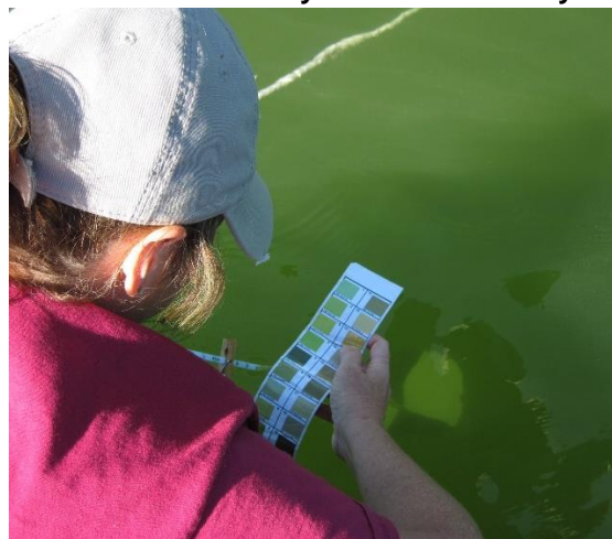
Figure 6. Volunteer Kristin Davis assesses water color by using a color chart held above her Secchi disk at Crystal Lake/McHenry Co.
