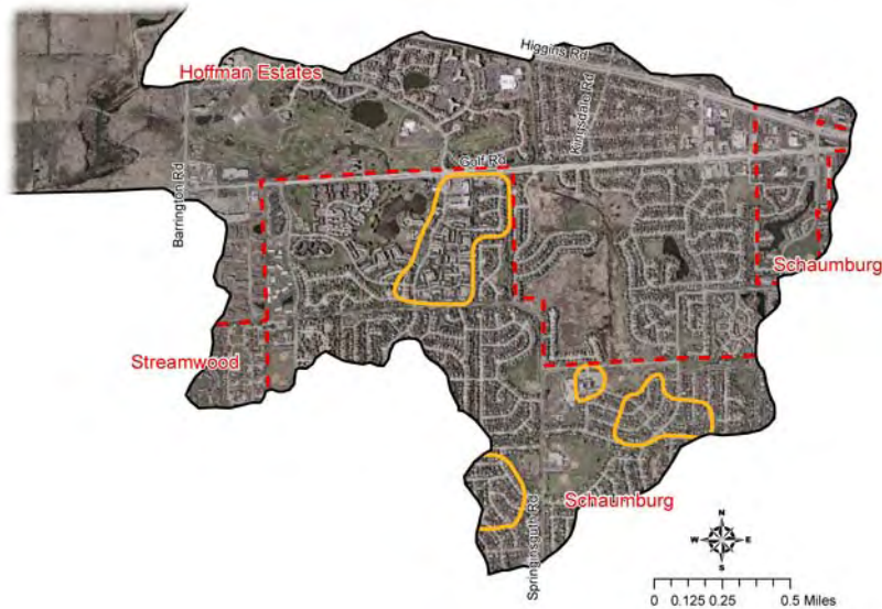
Figure 4-2. Approximate areas within Schaumburg in Subwatershed 500 not served by detention facilities.
