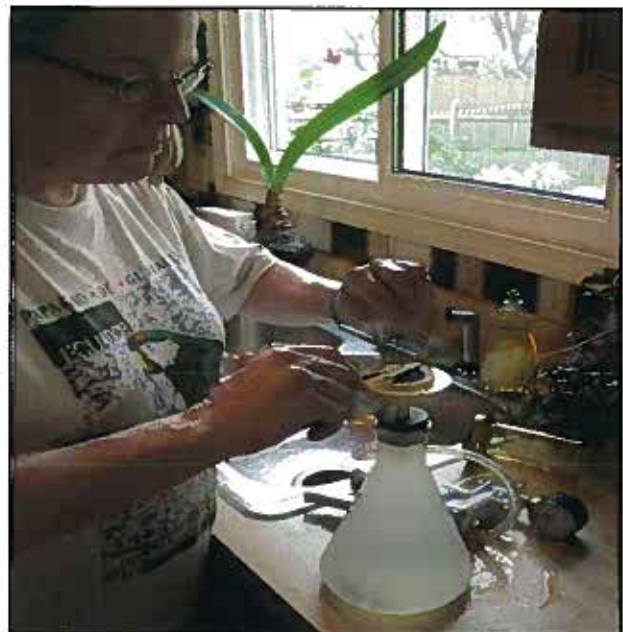
Volunteer Darlene Garay (Lake Charles, DuPage Co.) carefully folds a filter containing algae that will be shipped to an Illinois EPA laboratory for chlorophyll analysis.
