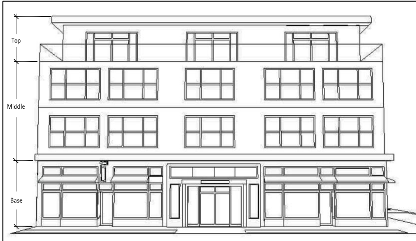
Articulated building with clearly defined base, middle, and top. (4.7.2.1)
