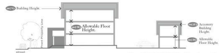
Figure N-2: Height & Use Requirements.
