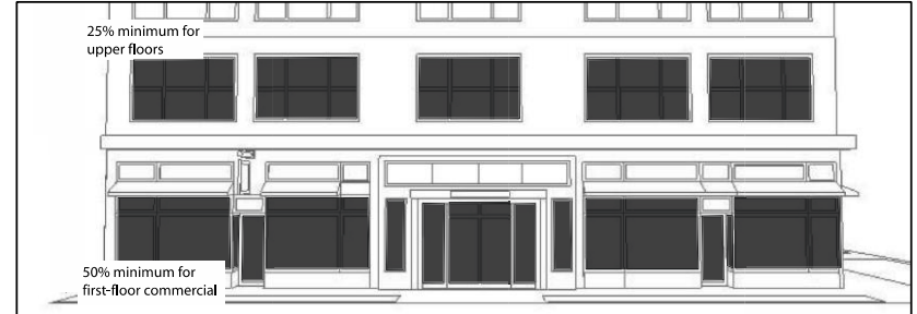
At least 50% of ground-floor commercial shall be clear glass windows and doors. At least 25% of every upper floor shall be glass windows. (4.7.4.3, 4.7.4.4)
