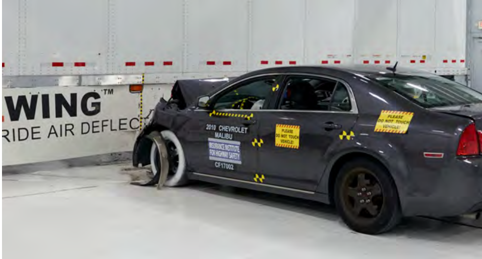
Figure 2: In a simulation, a side guard stopped the car from going underneath the trailer. Image credit: IIHS, May, 2017.
